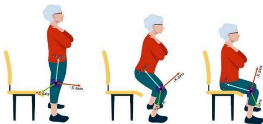
Figure 2. IMU Position in Sit and Stand Task
